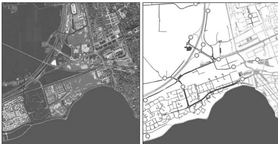
Fig. 6 Accessibility of roads—another map resulting from the system that shows the mitigation of the flood (left) and the road access in the study area (right) accordingly. In the access map (right), green paths show usable road paths while red-circled icons symbolize access bottlenecks
